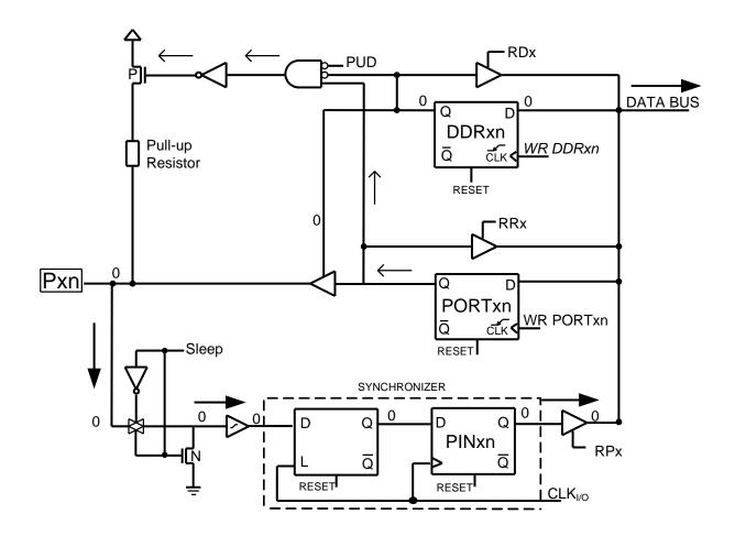
The  $\leftarrow$  represents how the content of PORTx register affects the pull-up resistor; while the  $\rightarrow$  shows how a data can be read from a pin
